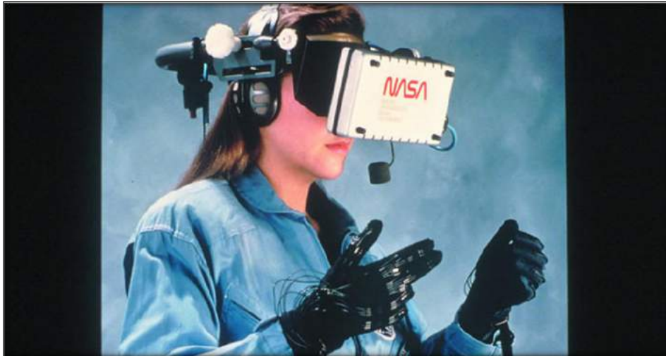
Fig. 9: VPL power gloves in NASA. Source: (BARNARD, 2019).
